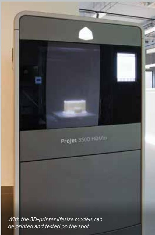
With the 3D-printer lifesize models can be printed and tested on the spot.
